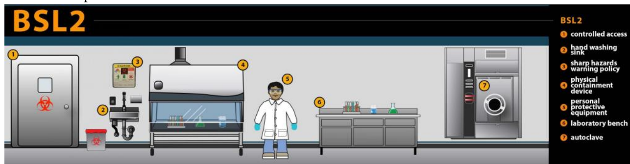
Figure 49. Biosafety Level 2 (BSL-2) Infographic. Source: Centers for Disease Control and Prevention. 4 Biosafety Levels (cdc.gov)
